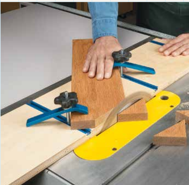
▲ Accurate Angles. Remove the fence and use the hold-downs to make steeper angle cuts.
