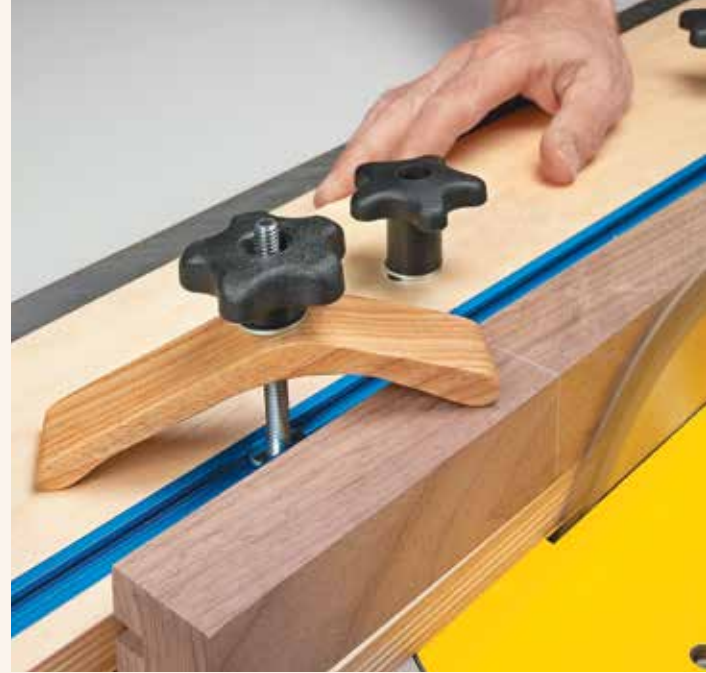
▲ A Firm Grip. In just a few minutes, you can make a hardwood hold-down. It locks a workpiece in place with the simple turn of a knob.
