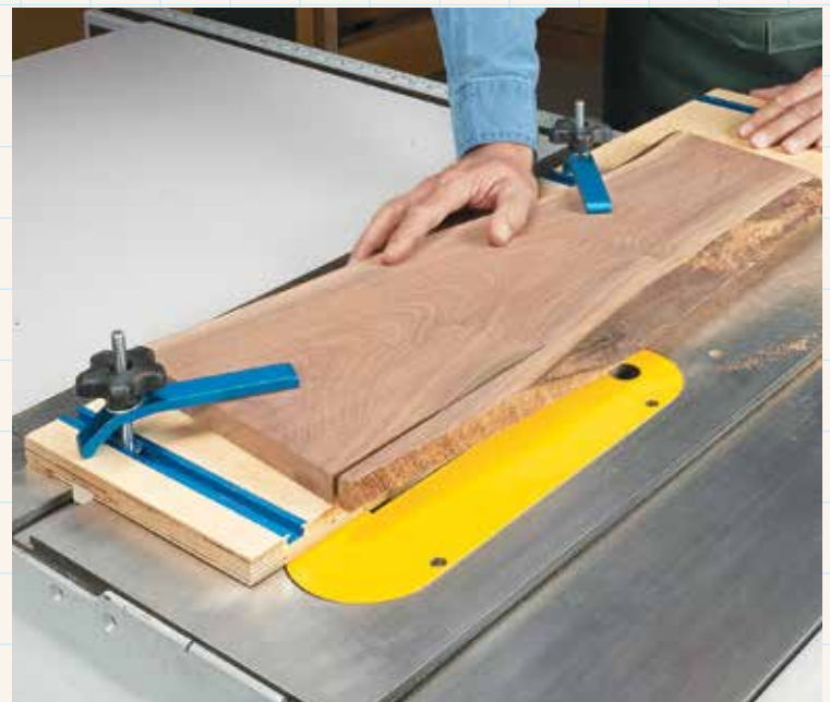
▲ Get a Straight Edge. You can secure rough-edged lumber to the base and rip a straight edge safely and easily.
