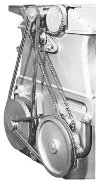
Illustration above shows two rear guards removed giving easy access to feed and cutterblock drives. The drive to the cutterblock is by twin space-saver vee belts. The chain drive to the feed passes over the chain tensioning sprocket and is driven direct from the gear box.
