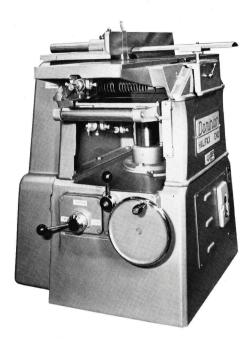
Illustration above shows centre column carrying bottom table, handwheel for raising or lowering bottom table and gear lever for feed speeds. Also illustrated is the small handwheel adjustment for simultaneous raising or lowering of the bottom table rollers - an unusual feature on a machine of this capacity.
